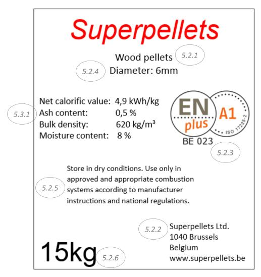
Figure 1: Illustration of a bag design
