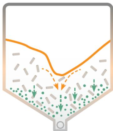
Consequence: The pellets in the lower area contain a lot of **fine particles**, which increase with each delivery when the storage is not completely emptied.
