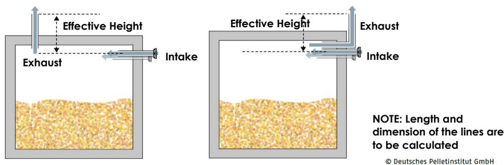
ISO standard 20023 also authorize solutions which consider the natural ventilation created by the difference of height between the higher-placed exhaust-air nozzle and the storage-side supply-air nozzle (see [Fig. 27](#)). The required height difference and the necessary cable diameter must be determined according to this standard.
