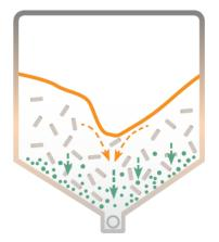
Consequence: The pellets in the lower area contain a lot of **fine particles**, which increase with each delivery when the storage is not completely emptied.
