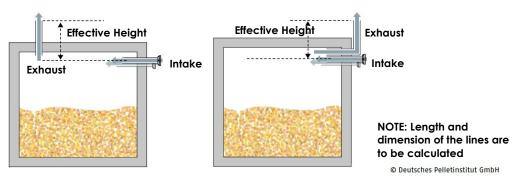
ISO standard 20023 also authorize solutions which consider the natural ventilation created by the difference of height between the higher-placed exhaust-air nozzle and the storage-side supply-air nozzle (see Fig. 27). The required height difference and the necessary cable diameter must be determined according to this standard.
