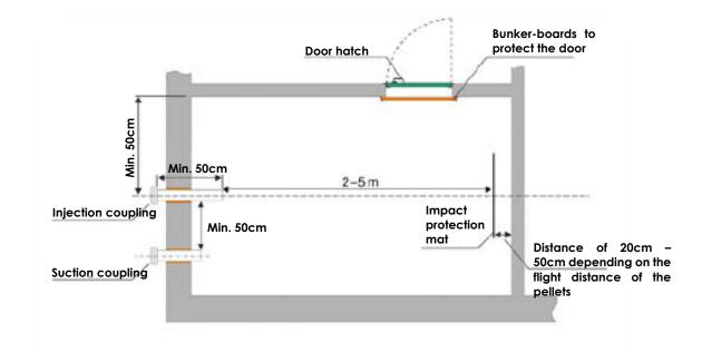
Floor plan of a pellet storage room (ventilation via filling system)
